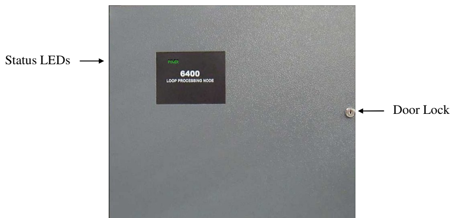
FIGURE 2 - Loop Processing Node (LPN)
